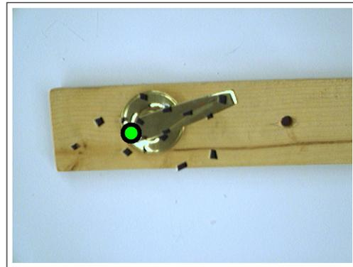
Fig. 6. The axis of rotation for a door knob, extracted using Interactive Perception.
