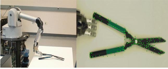
Fig. 2. *UMan* interacts with a tool by reaching its arm towards the tool. The right image shows the tools as seen by the robot, with dots marking the tracked features. The left image shows the experimental setting
